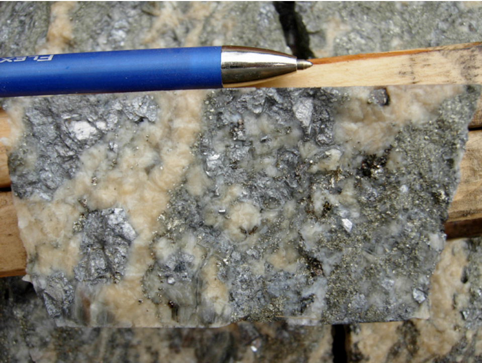
Figure 6. Rau property drill core (DDH08-05) with arsenopyrite, pyrite and pyrrhotite mineralization.
